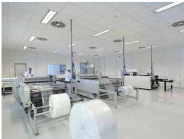
Fig. 3. Cleanroom production for manufacturing cleanroom packaging (© Strubl)
