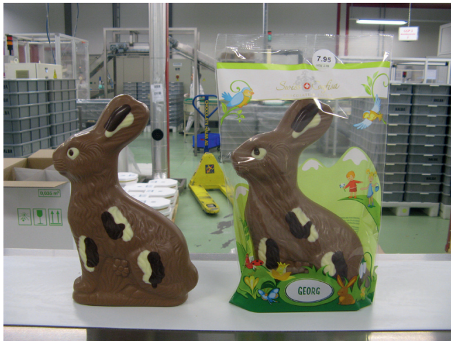
The pouches are made of OPP film (left). If large chocolate bunnies weighing 500 g are packaged, the system can run at up to 18 cycles/min.
