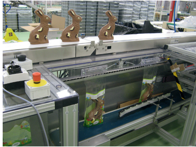
The pouches are made of OPP film (left). If large chocolate bunnies weighing 500 g are packaged, the system can run at up to 18 cycles/min.
